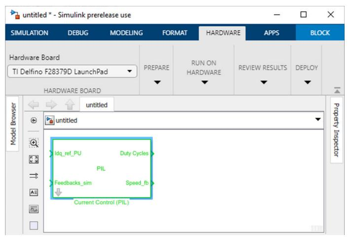
8 Copy the Current Control (PIL) subsystem and replace the Current Control subsystem in the mcb pmsm foc sim.slx example model.
