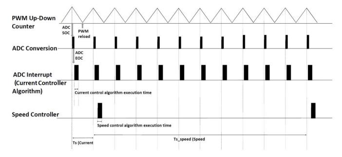
In this figure, the execution times for the current controller and speed controller are not in scale. See the processor datasheet to better understand the functionality of the processor peripherals such as the ADC (analog-to-digital converter) and the PWM (pulse-width modulation).
