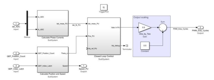
Add a Function-Call Generator block from the Simulink/Ports & Subsystems library to the subsystem created in step 5. Set the **Sample time** parameter of the block to equal the control-loop sample time,  $T_s$  (that has a default value of 50e-6 s).
