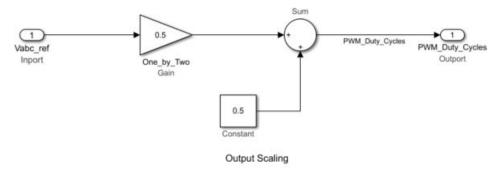
Create a new subsystem by integrating the current scaling (Calculate Phase Currents), QEP position decoding (Calculate Position and Speed), Closed Loop Control, and Output Scaling subsystems. Add the Trigger block from the Simulink/Ports & Subsystems library to this subsystem and set the **Trigger type** parameter to function-call.
