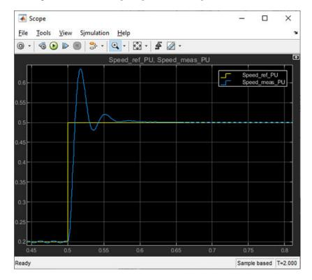
This procedure shows a method to implement speed control for a PMSM in simulation. Run the simulation and analyze the controller performance.
