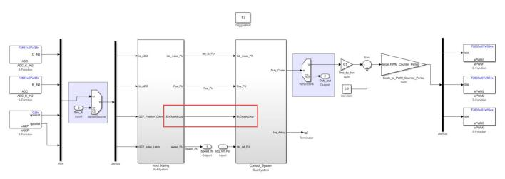
4 Copy the mcb\_pmsm\_foc\_qep\_f28379d/Speed Control/Speed\_Ref\_Selector subsystem to your model and integrate it with the speed controller subsystem. When the closed-loop control begins, this subsystem provides the Speed\_Ref ouput signal. For a smooth transition from open-loop to closed-loop, the speed measured is used as the speed reference during the open-loop run. Add a Data Store Write block SpeedRef to the PI\_Controller\_Speed input port.
