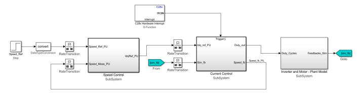
In the Rate Transition block input to Current Control subsystem, change the **Output port sample time** to -1.
