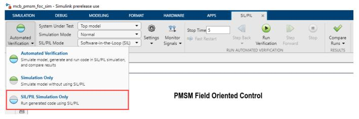
12 Select Model blocks in SIL/PIL mode in the System Under Test field.
