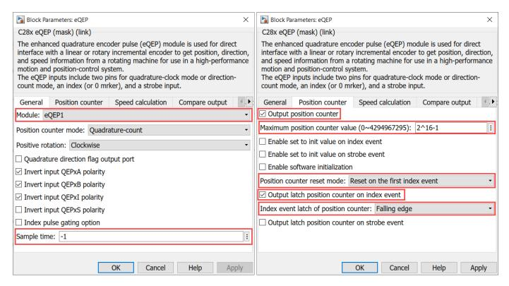
eQEP1 module is selected because the quadrature encoder is connected to the QEP\_A interface on the LaunchPadXL28379d hardware board. The sample time is -1 because the library block is function-call triggered by the ADC interrupt synchronously. The maximum position counter value is 2^16-1 because the position counter uses a 16-bit architecture in the library driver block. The position counter reset mode setting wraps the position count when the index pulse is read.
