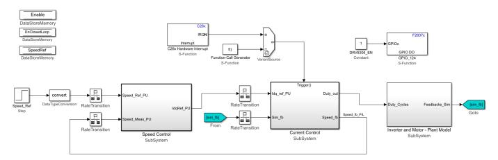
On the **Hardware** tab of the Simulink model, select **Build, Deploy & Start**. This generates the C code, CCS project, and a target-specific .out file. The system uses serial communication to download this target specific .out file to the target hardware and runs the downloaded algorithm in the hardware.
