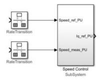
Integrate the speed controller subsystem (that you created in step 2) with the integrated current controller and plant model subsystems. Connect the **Iq\_ref\_PU** output port of the speed
