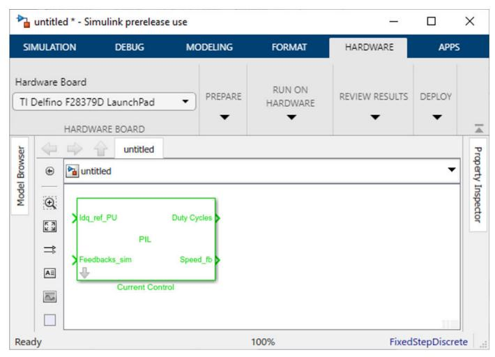
**7** Rename the Current Control subsystem to Current Control (PIL).
