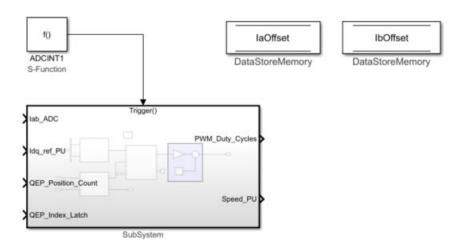
7 Integrate the plant model and the controller subsystem that you created in step 6. For detailed steps on how to create a plant model for a motor control system, see "Creating Plant Model Using Motor Control Blockset" on page 3-2.
