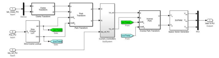
Integrate the components that you created in step 2 into a single subsystem (Closed Loop Control that implements closed loop field-oriented control) as shown in this figure.
